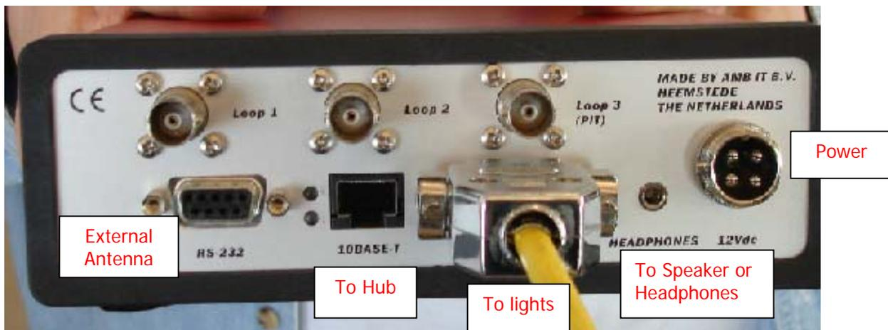
Picture 4 Decoder – only Photocell Cable connected. Note Loop3 for Pit ONLY
